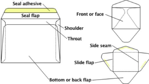
The envelopes with the opening and seal flap located on the short dimension are called Open End envelopes. Those with the flap on the short dimension are called Open Side envelopes. Such envelopes are ideal for automatic insertion applications.
